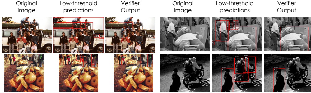
Figure 12: Failure cases of our VLM-based verifier. For each sample we show the original image, the predicted bounding boxes by the low-threshold model, and the final pseudo-annotations produced by the VLM verifier. Our verifier occasionally fails when two similar objects overlap significantly.
