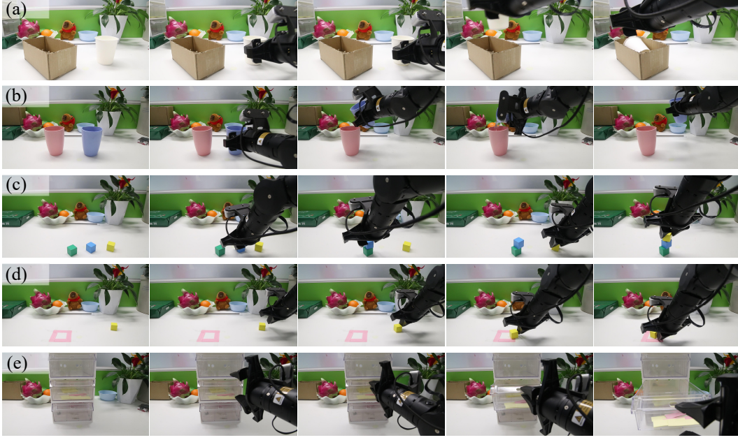
Figure 10: Visualization of general tasks. (a) Bottle pick and place. (b) Liquid pouring. (c) Stacking cubes. (d) Push-to-position. (e) Opening a drawer.
