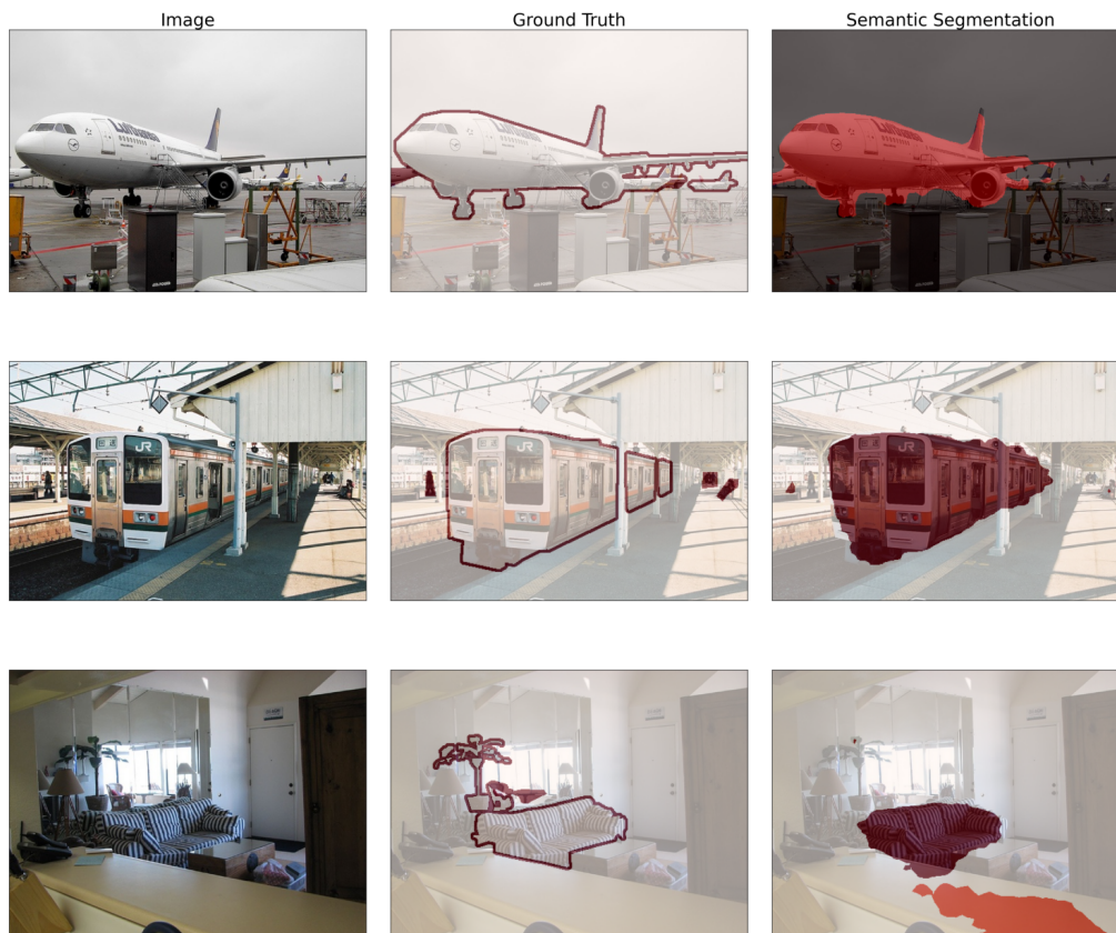
Figure 1: Example Outputs of Semantic Segmentation Featuring Noticeable Irregular Masks. From left to right: Original image, Ground truth, Deeplab output.
