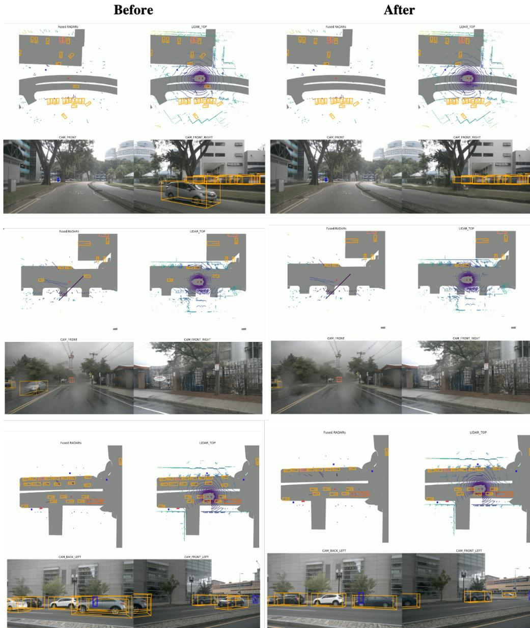
Figure 7: Examples with deleting moving vehicles. Visualized along with annotations.
