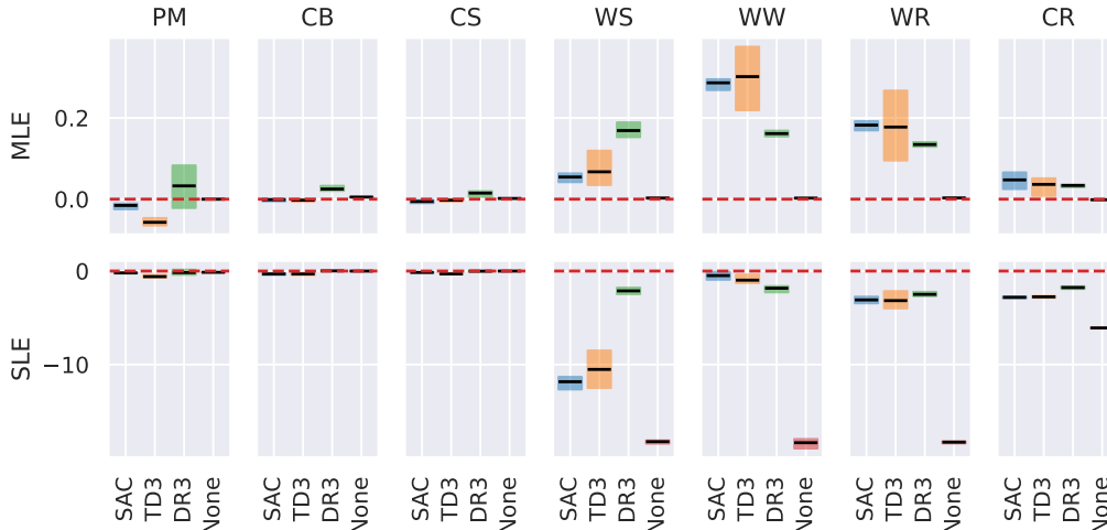
Figure 3: Estimated Maximal Lyapunov Exponent (MLE) and Sum of Lyapunov Exponents (SLE) for the Pointmass (PM), Cartpole Balance (CB), Cartpole Swingup (CS), Walker Stand (WS), Walker Walk (WW), Walker Run (WR) and Cheetah Run (CR) environments when controlled by a trained instance of SAC, TD3, Dreamer V3 (DR3) and an agent which takes no actions (None). Each policy-environment combination is independently trained with three random seeds and the interquartile average MLE & SLE for each seed is calculated using 20 initial states. A bootstrapped 95% confidence interval is included to show the variation in MLE and SLE across random seeds.
