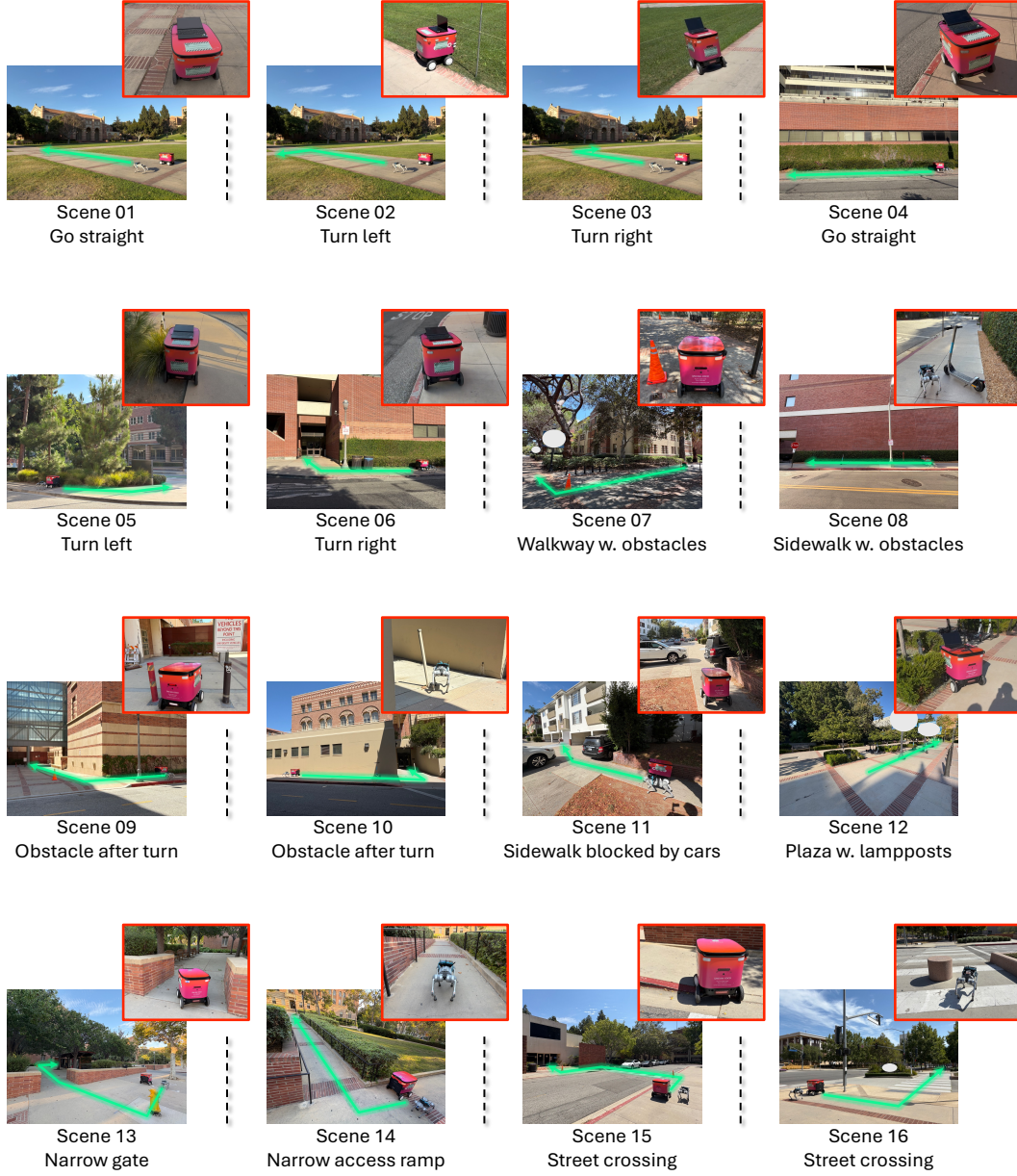
Figure 23: Real-world testing scenarios. We evaluate zero-shot sim-to-real policy transfer across 16 diverse urban scenes and two embodiments (COCO wheeled delivery robot and Unitree Go2 quadruped), spanning challenges such as straight paths (Scenes 01, 04) and turns (Scenes 02, 03, 05, 06) on open ground or sidewalks, walkway and sidewalk obstacles (Scenes 07, 08), obstacles appearing after turns (Scenes 09, 10), sidewalk blockage by cars (Scene 11), structural elements including lampposts and narrow access points (Scenes 12–14), and street crossings (Scenes 15, 16). Key challenges for each scene are highlighted in Red at the upper-right corner.
