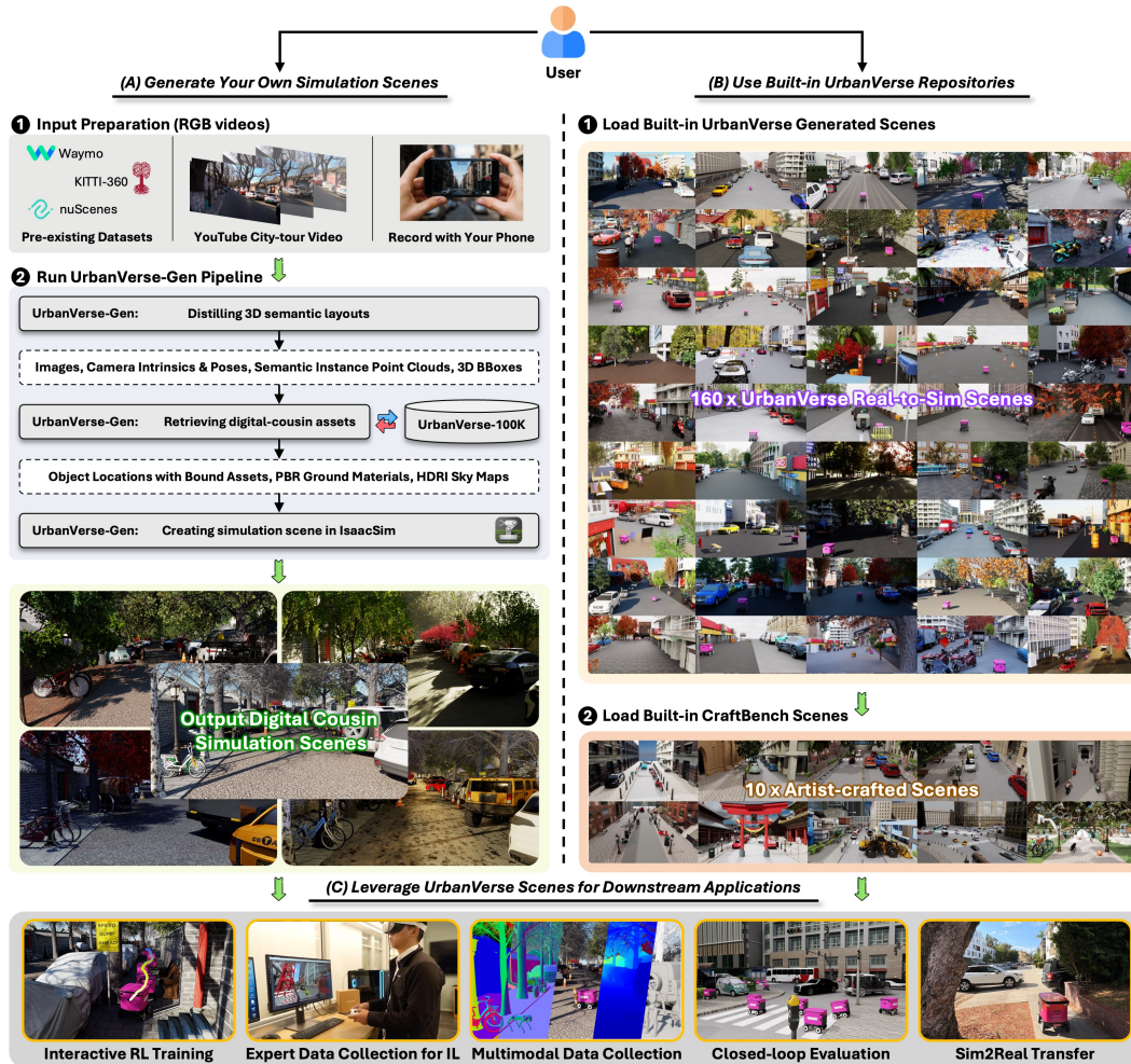
Figure 12: User-side pipeline of the UrbanVerse simulation platform.
