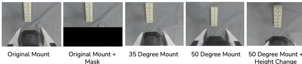
Figure 13: **Our wrist camera viewpoints.** This figure depicts the viewpoints we used for our ablations. The lego block is in the same place directly under the gripper for all mounts. Different wrist camera angles can cause the same object to appear in different parts of an egocentric image.
