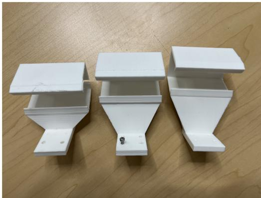
Figure 12: **Our wrist camera mounts.** The follow depicts the original, 35-degree and 50-degree mounts.
