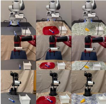
Figure 3: **Pick/Place Tasks.** The left column contains the shared pick/place task, while the other columns contain the new distractor and new object variants. For zero-shot evaluation, we include data for the shared task across all robots. For few-shot, we also include 5 demonstrations of a variant for one robot.
