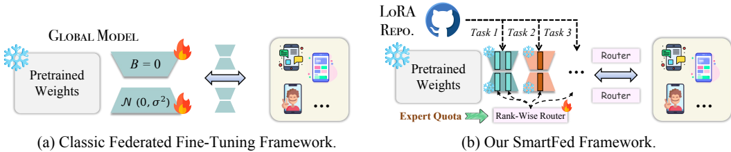
Figure 1: Illustration of the classic federated fine-tuning framework versus our SMARTFED. Classic methods train LoRA modules from scratch (a), while SMARTFED updates only the router (b).
