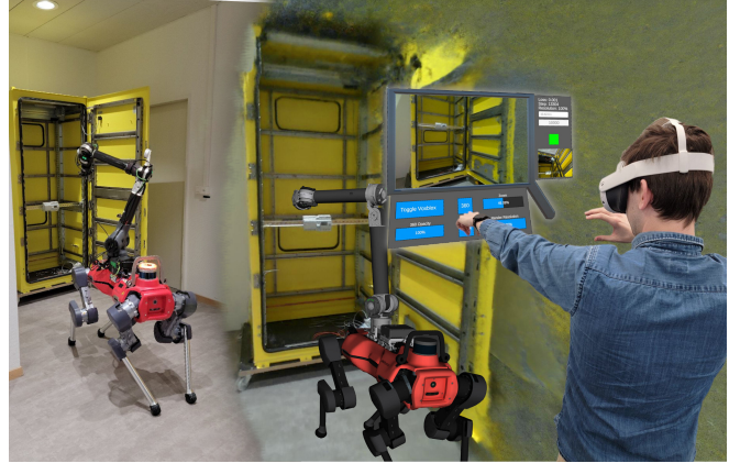
Fig. 1. Teleoperator controlling a robot using a VR interface from inside a reconstructed Radiance Field. Reconstructions are created online from any robot based on its sensor configuration. Neural Radiance Field or Gaussian Splatting renders can be displayed in an immersive 360° render or on a handheld viewer. These renders are displayed alongside the robot and its sensor data, such as camera feeds and LiDAR.
