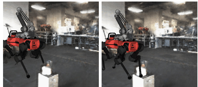
Fig. 4. Sample of the RViz plugin occluding the robot based on scene depth (left) and having the robot rendered on top (right).
