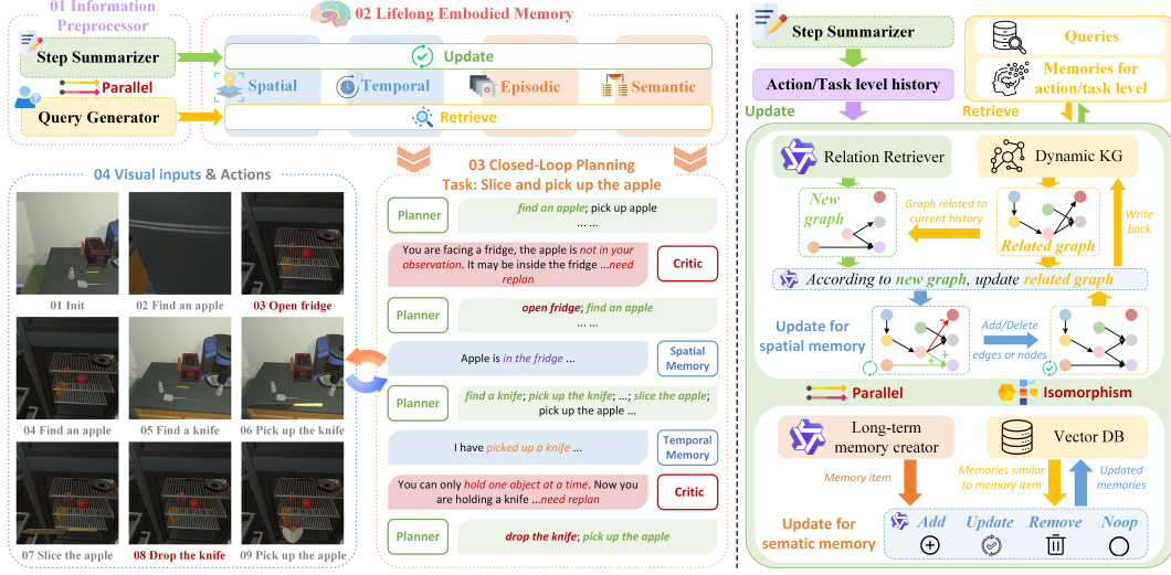
Figure 2: RoboMemory architecture with working pipeline and memory mechanisms. (a) Left: The agent’s pipeline. Parallel Step Summarizer and Query Generator in Information Processor (1) generate updates/queries for Lifelong Embodied Memory (2). These memories enable Closed-Loop Planning (3) for tasks like “slice and pick up the apple”—the Planner generates plans, while the Critic and memories adjust decisions via feedback from visual inputs/results (4). (b) Right: Spatial and Semantic memories operate in parallel with isomorphic updates. Internally, Spatial memory maintains a relevance/similarity-updated KG, and Semantic memory manages a Vector DB with analogous logic.
