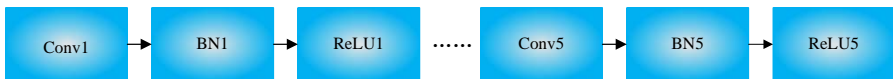
Figure 2: The first five convolutional layers of our proposed model. The batch normalization (BN) layer is placed between each convolutional layer (Conv) and the succedent ReLU layer. In the first two convolutional layers, the max-pooling layer is placed to follow the ReLU layer.
