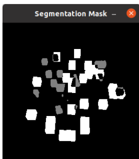
Figure 3: The goal mask not reached is the same as the error mask reached. The gray box is the mask at the wrong position, and the white box is the target position not reached
