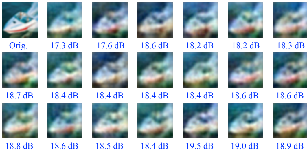
Figure 24: Example 4: Impact of output channel selection on the quality of reconstructed images, m = 6 , D' = 16 .
