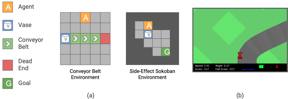
Figure 2: (a) The gridworld environments are specifically designed to test agents against negative side effects. Usage of imaginative module ensures that the agent does not take actions which lead to negative side effects in the future. (b) The car simulator environment used to train the agent to drive safely without going off the track. The baseline states here represents unsafe states.
