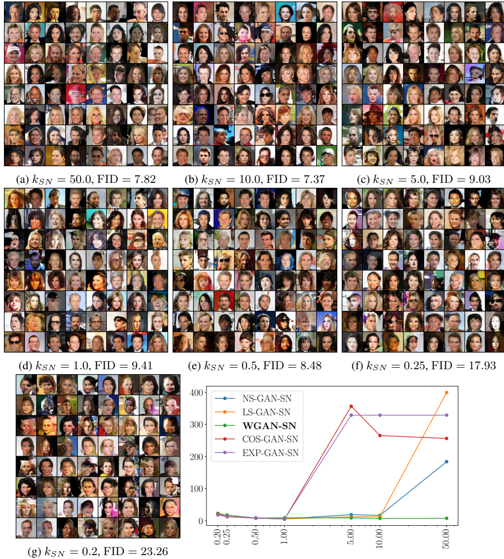
Figure 16: Samples of randomly generated images with WGAN-SN of varying k_{SN} (CelebA). For the line plot, x -axis shows k_{SN} (in log scale) and y -axis shows the FID scores.
