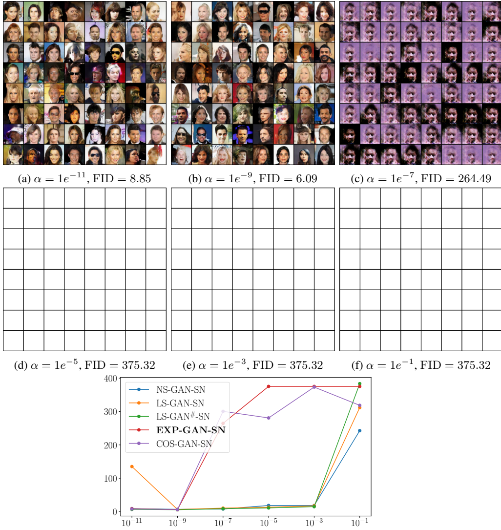
Figure 32: Samples of randomly generated images with EXP-GAN-SN of varying \alpha ( k_{SN} = 50.0 , CelebA). For the line plot, x -axis shows \alpha (in log scale) and y -axis shows the FID scores.
