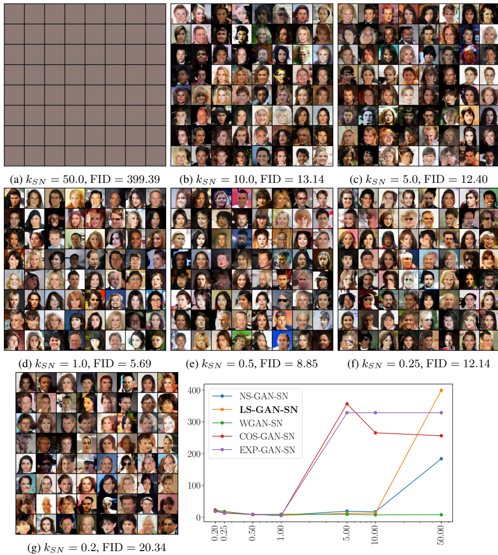
Figure 15: Samples of randomly generated images with LS-GAN-SN of varying k_{SN} (CelebA). For the line plot, x -axis shows k_{SN} (in log scale) and y -axis shows the FID scores.
