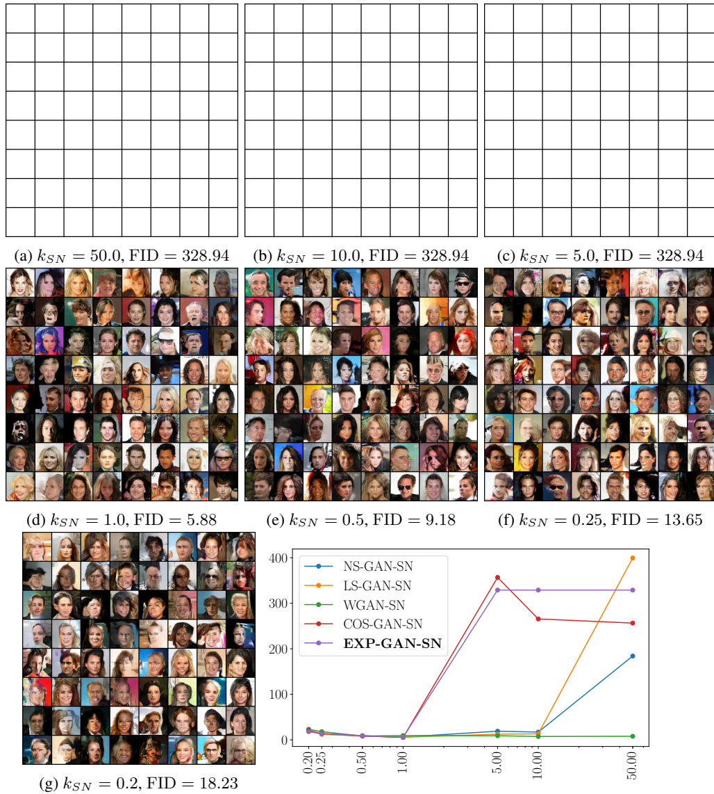
Figure 18: Samples of randomly generated images with EXP-GAN-SN of varying k_{SN} (CelebA). For the line plot, x -axis shows k_{SN} (in log scale) and y -axis shows the FID scores.
