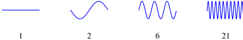
Figure 3: The 1st, 2nd, 6th, and 21th trigonometric basis functions in dimension n = 300 .
