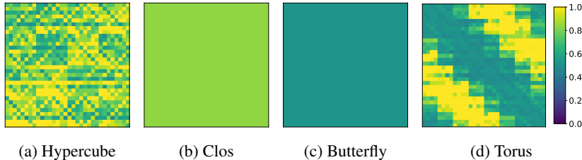
Figure 5: Controllability matrix K after 1000 training iterations. All networks have 32 inputs and outputs, and 1152, 1152, 1152, and 1120 edges, respectively. Clos router configuration is (8, 9, 8), hypercube has 6 layers, butterfly has 18 layers, and the torus has 8 rows and 4 columns.
