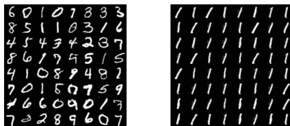
Figure 9: Images generated by a basic GAN on MNIST before and after mode collapse. The left image shows GAN-produced images early in GAN training and the right image shows GAN samples later in training after mode collapse has occurred due to training instabilities.
