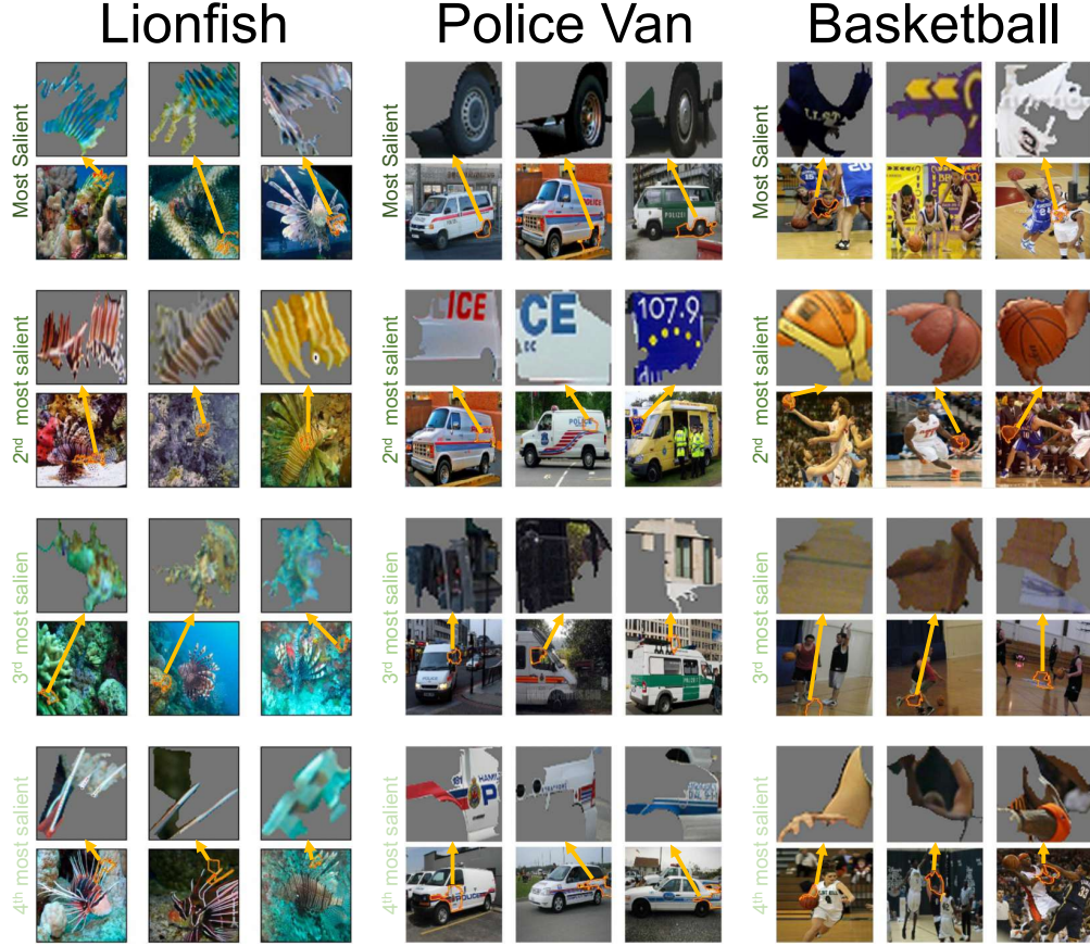
Figure 2: The output of ACE for three ImageNet classes. Here we depict three randomly selected examples of the top-4 important concepts of each class (each example is shown above the original image it was segmented from). Using this result, for instance, we could see that the network classifies police vans using the van’s tire and the police logo.
