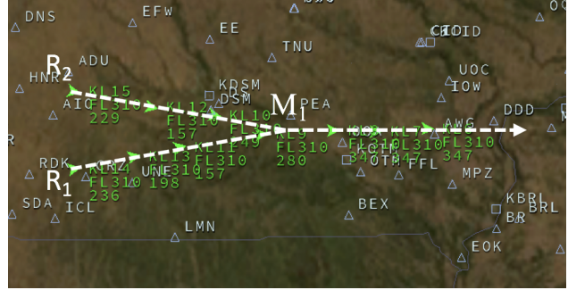
Figure 4. Case Study 2: two routes, R_1 and R_2 merge to a single route at M_1 .
