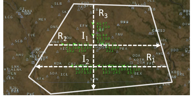
Figure 2. BlueSky sector designed for our Case Study. Shown is Case Study 1 for illustration: there are three routes, R_1 , R_2 , and R_3 , along with two intersections, I_1 and I_2 .
