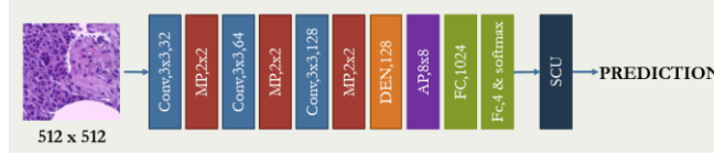
Figure 5: The architecture of proposed deep learning framework. DEN is the Deep Extraction Network module, and SCU is the Slice-base Classification Unit.
