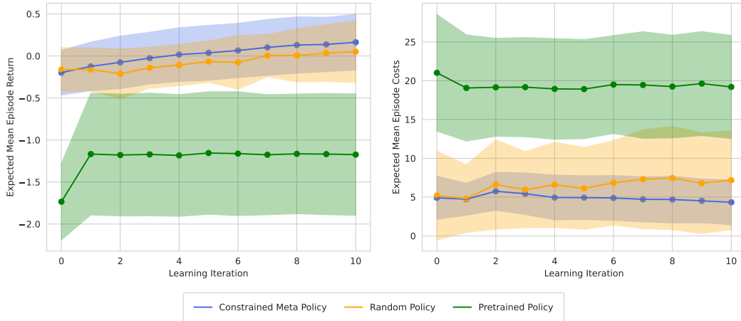
Figure 10: Progression of the mean episode returns and mean episode costs throughout the fine-tuning process. In contrast to Figure 4, an average has been computed across the means of three different seeds, along with the indication of the mean standard deviation of these three seeds. The constrained meta-policy has undergone meta-training using TRPOLag. In fine-tuning, all policies have been adjusted with TRPOLag.
