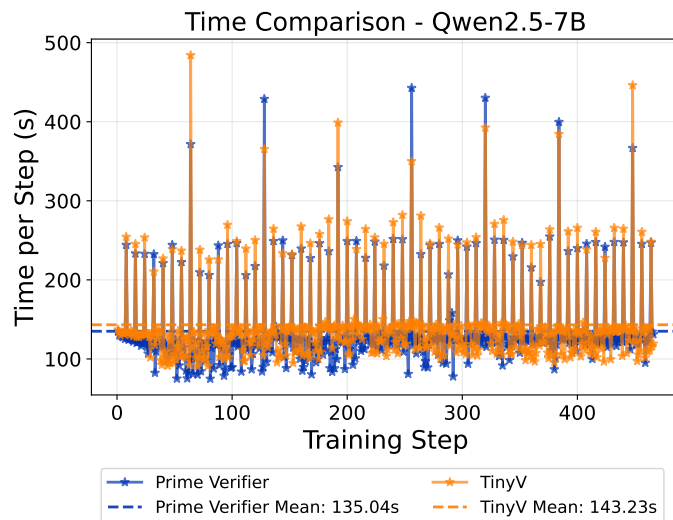
Figure 12: This figure compares the average time cost of TINYV with Prime Verifier during GRPO training. The peak occurs when saving model checkpoints.
