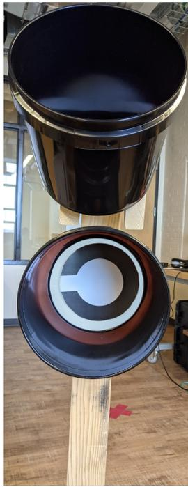
Fig. 5. A view of the lower Landolt C vision acuity test on a navigation goal.
