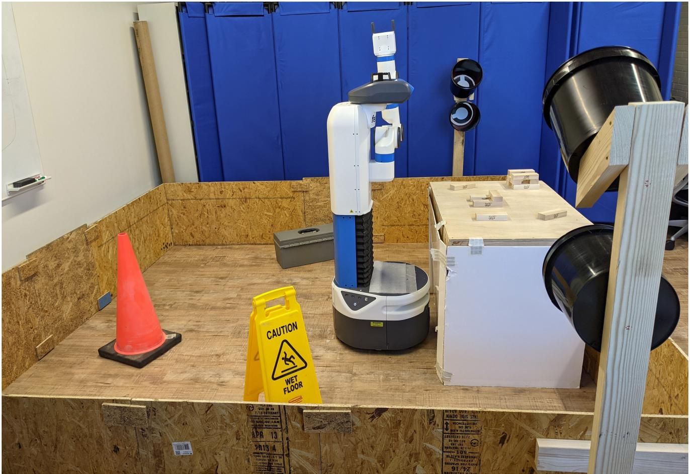
Fig. 3. The arena used in this user study. Here you can see the three obstacles for the navigation task including a traffic cone, wet floor sign, and toolbox. On the right side of the image you can see two of the navigation goals each with two buckets containing a Landolt C visual acuity chart. Lastly, in front of the robot you can see the table used for the manipulation block stacking task.
