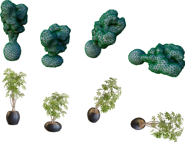
Fig. 10. The NeRF ficus undergoing elastic deformation. Top row : Simplified view of the tetrahedral cage surrounding the density mesh extracted from the static scene. Bottom row : Rendered result. Best viewed zoomed in.
