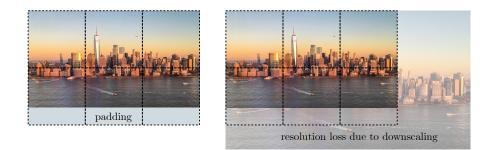
Figure 11: Illustration of image grid selection used in dynamic image splitting for high-resolution image encoding. (Left) If the grid can cover the full image without scaling down, we choose the grid that minimizes padding. (Right) Otherwise, we choose the grid that minimizes the resolution loss due to scaling down.
