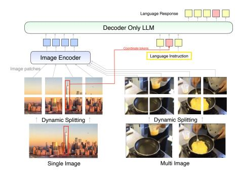
Figure 12: The overview of model architecture. MM1.5 excels at (*i*) text-rich image understanding with dynamic image splitting, (*ii*) visual referring and grounding with coordinate tokens, and (*iii*) multi-image reasoning.
