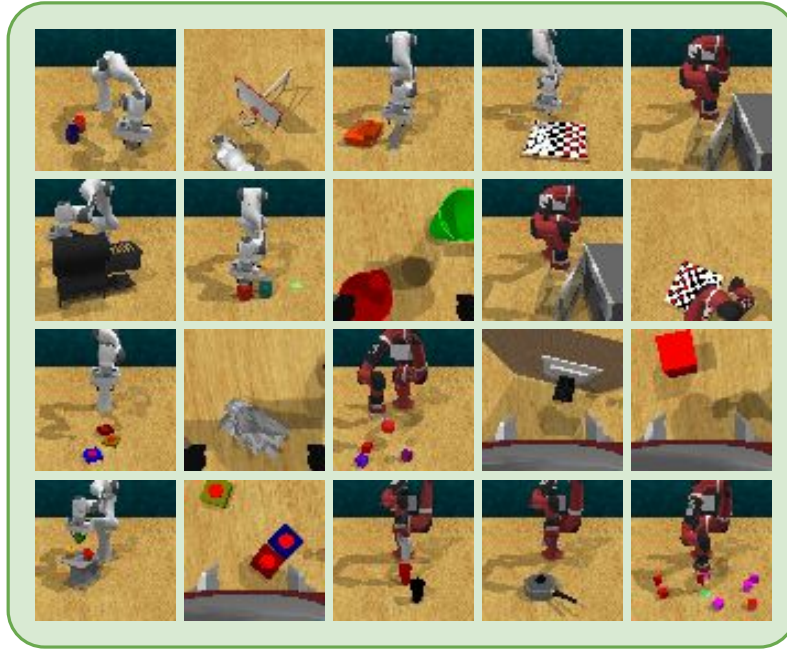
Figure 15: A single autoregressive video model is trained on 30 tasks for the Franka Panda and 23 tasks for the ReThink Robotics Sawyer, using 16 \times 16 VQCodes and a context length of 4, with frame skip 4.
