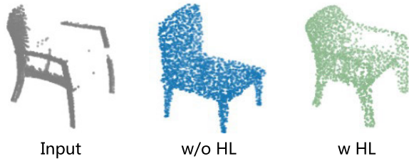
Fig. 3. Illustration of the impact of the HL loss. With a GAN loss, only the general shape of a category can be predicted. The HL loss can adjust the general shape of a category to a specific 3D shape that is as similar as possible to the input partial object.
