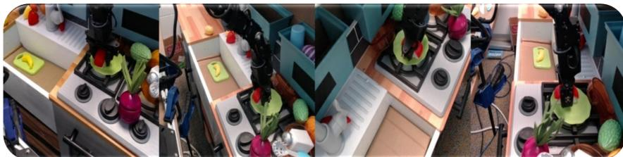
Figure 24: A sample frame of BridgeData V2 dataset presented in 1 to 4 exocentric views used in the ablation study to examine the effects of richer visual information
