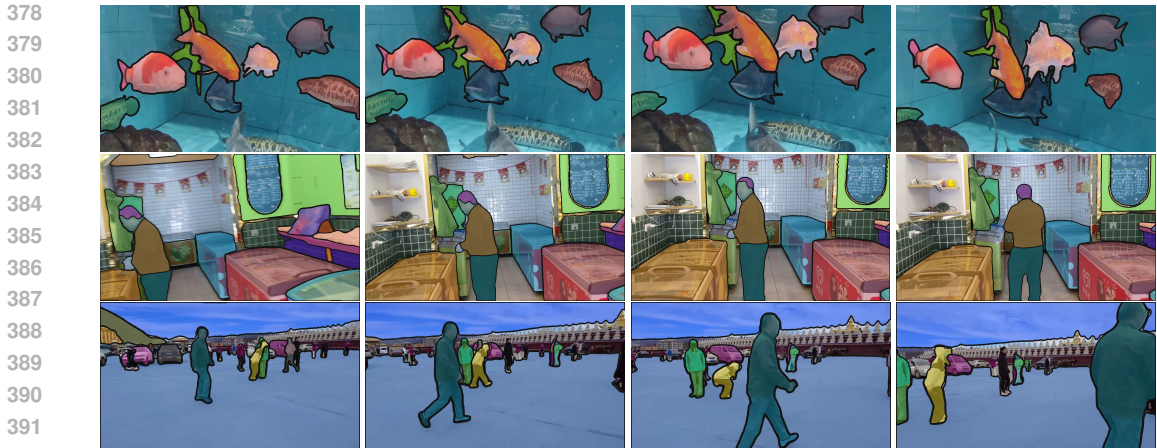
Figure 4: Example videos from the SA-V dataset with masklets overlaid (manual and automatic). Each masklet has a unique color, and each row represents frames from one video, with 1 second between them. More examples in Fig. 11.
