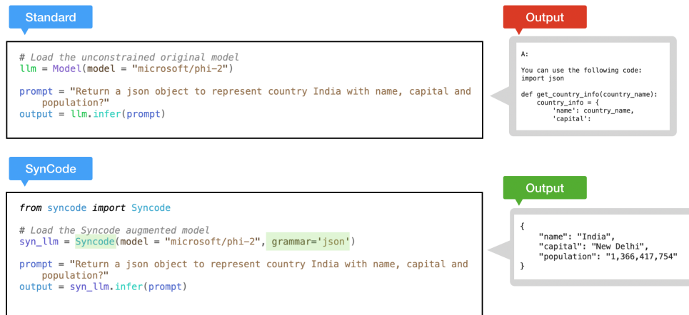
Figure 9: The upper section displays erroneous output from a standard LLM generation, failing to produce the intended JSON format. The lower segment showcases the fix achieved through the use of the SYNCODE framework.
