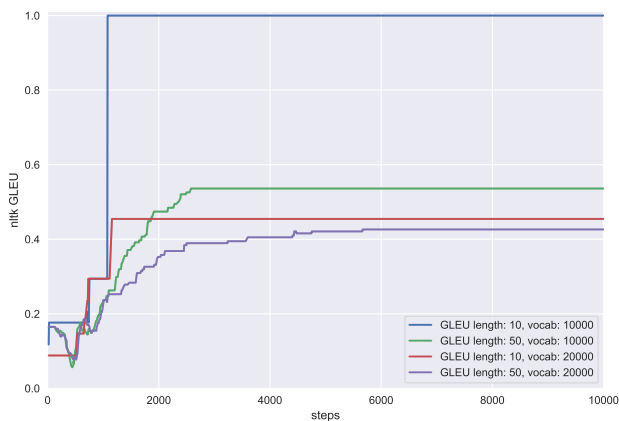
Figure 2: GLEU score during training of the model trained on the GLEU loss with different sequence lengths and vocabulary sizes.
