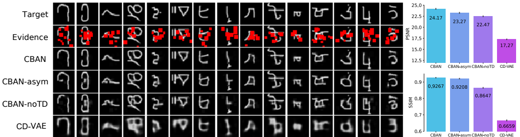
Figure 5: Omniglot image completion comparison examples (left) and quantitative results (right). The top two rows of the examples show the target image and the evidence provided to the model (with missing pixels depicted in red), respectively. The subsequent rows show the image completions produced by CBAN, CBAN-asym, CBAN-noTD, and the denoising VAE. The quantitative measures evaluate each model on PSNR and SSIM metrics; black lines indicate +1 standard error of the mean.
