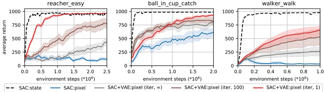
Figure 2: Separate  $\beta$ -VAE and policy training with no shared gradients SAC+VAE:pixel (iter,  $N$ ), with SAC:state shown as an upper bound.  $N$  refers to frequency in environment steps at which the  $\beta$ -VAE updates after initial pretraining. More frequent updates are beneficial for learning better representations, but cannot fully address the gap in performance. Full results in Appendix C.
