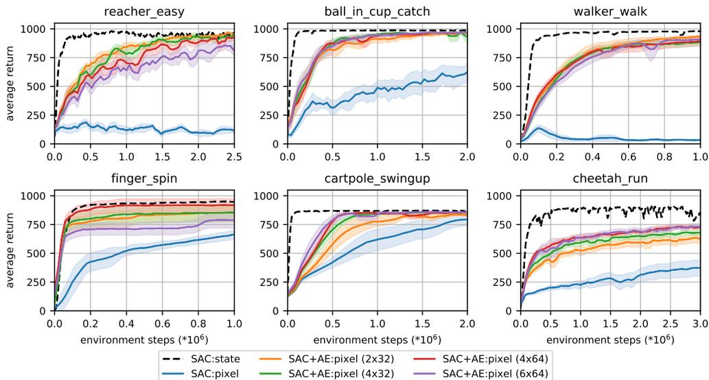
Figure 11: Different autoencoder architectures, where we vary the number of conv layers and the number of output channels in each layer in both the encoder and decoder. For example,  $4 \times 32$  specifies an architecture with 4 conv layers, each outputting 32 channels. We observe that the difference in capacity has only limited effect on final performance.
