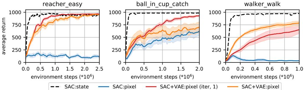
Figure 3: An unsuccessful attempt to propagate gradients from the actor-critic down to the encoder of the  $\beta$ -VAE to enable end-to-end off-policy training. The learning process of SAC+VAE:pixel exhibits instability together with the subpar performance comparing to the baseline SAC+VAE:pixel (iter, 1), which does not share gradients with the actor-critic. Full results in Appendix D.
