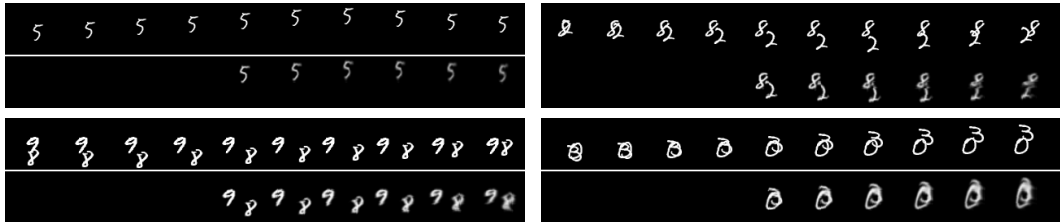
Figure 4: Predictions of 4 sequences from the moving MNIST dataset. The top row of each pair shows the ground truth frames; the first four frames are used as input to the model. The bottom row shows the predictions of the model.
