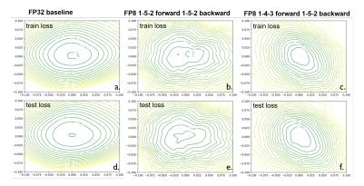
Figure 3: The loss surfaces of models trained in different precisions: (a) FP32, (b) FP8 (all GEMMs in 1-5-2, [2]), (c) HFP8 (1-4-3 only for forward pass). The top row for the loss surfaces from training data while the bottom row from test data. The loss surfaces with HFP8 maintain good Lipschitz properties compared to FP32 while the loss surfaces with FP8 exhibit multiple saddle points which hinder training convergence.
