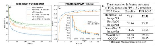
Figure 1: Challenges in the previous FP8 (1-5-2) format. (a) FP8 training on MobileNetV2 with different width multipliers—showcasing significant accuracy degradation from FP8 training for capacity constrained models. (b) FP8 training on Transformer-based machine translation — large loss in BLEU scores. (c) Table for Trans-Precision inference from FP32 to FP8 — large accuracy loss observed in various domains.
