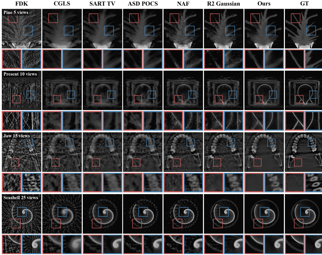
Figure 3: Qualitative evaluation of reconstruction algorithms under varying degrees of data sparsity. Our coarse-to-fine approach uses a 3D volumetric error map to strategically allocate model capacity, focusing refinement only on regions with high structural error. This targeted strategy avoids overfitting to sparse views, resulting in a cleaner and more geometrically accurate reconstruction. Zoomed-in patches are provided for a clearer inspection of reconstruction quality.
