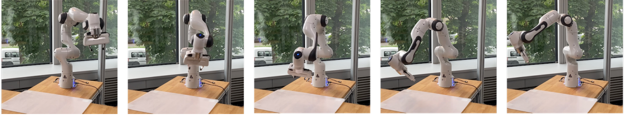
Figure 12: Real-world Franka trajectory. Example of a real-world trajectory of the Franka Panda robot arm, controlled by MELRO. The movement took approximately five seconds.
