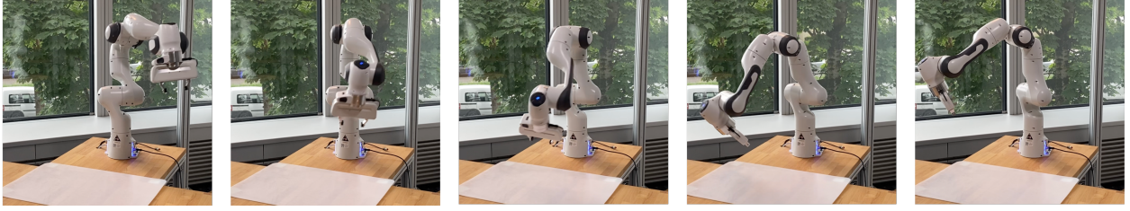
Figure 7: Franka Trajectory. Example of a real-world trajectory of the Franka Panda robot arm, controlled by MELRO. The movement took approximately five seconds.
