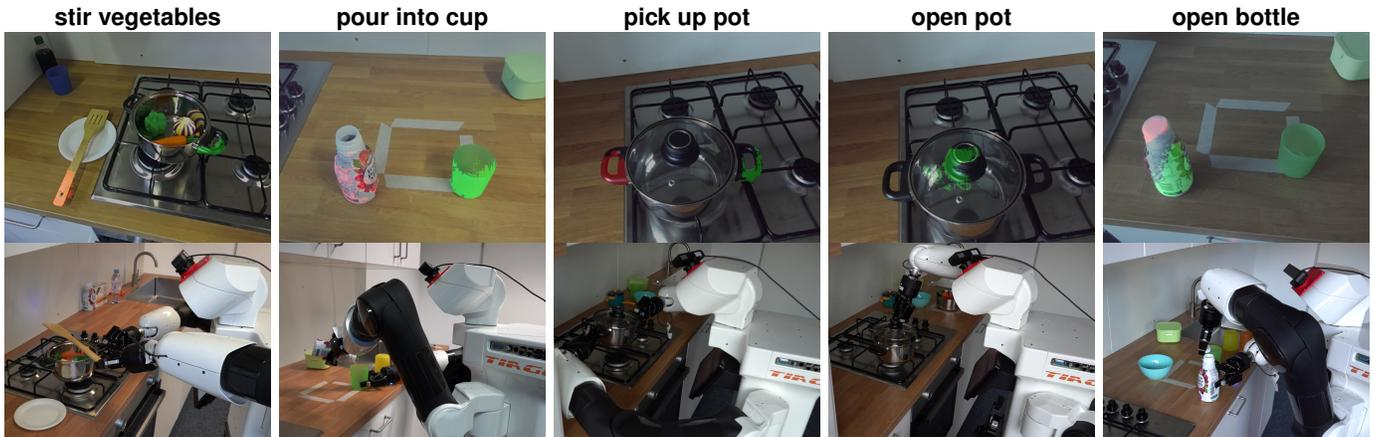
Fig. 6: Examples of different manipulation tasks executed on a bimanual Tiago++ robot. Red and green masks denote left and right hand affordance mask predictions, respectively. We segment the task-specific object affordance regions, propose grasps for these regions, and use pre-designed motion primitives to execute manipulation tasks.
