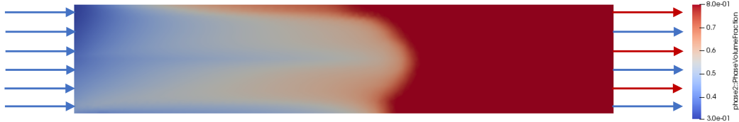
Figure 8: Two-dimensional homogeneous layered reservoir used for training. It shows the saturation of the displaced phase in one point in time during the numerical simulation. Blue represents the injected phase and red the displaced phase.
