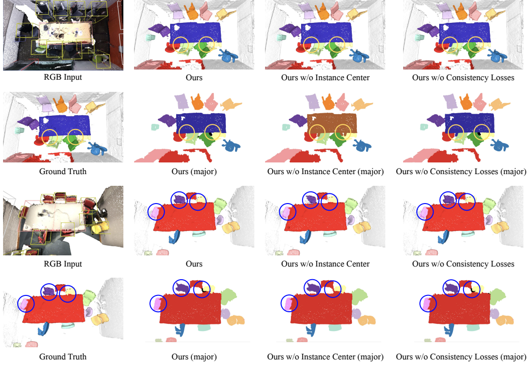
Figure A1: Qualitative comparison of model variants from the ablation study on ScanNetV2. Yellow boxes indicate ground-truth instance boxes, and circles highlight overlapping regions. Each row includes the RGB input, ablated model predictions, the ground truth, and an additional visualization highlighting only the predicted mask with the highest IoU(major) for each ground-truth instance.
