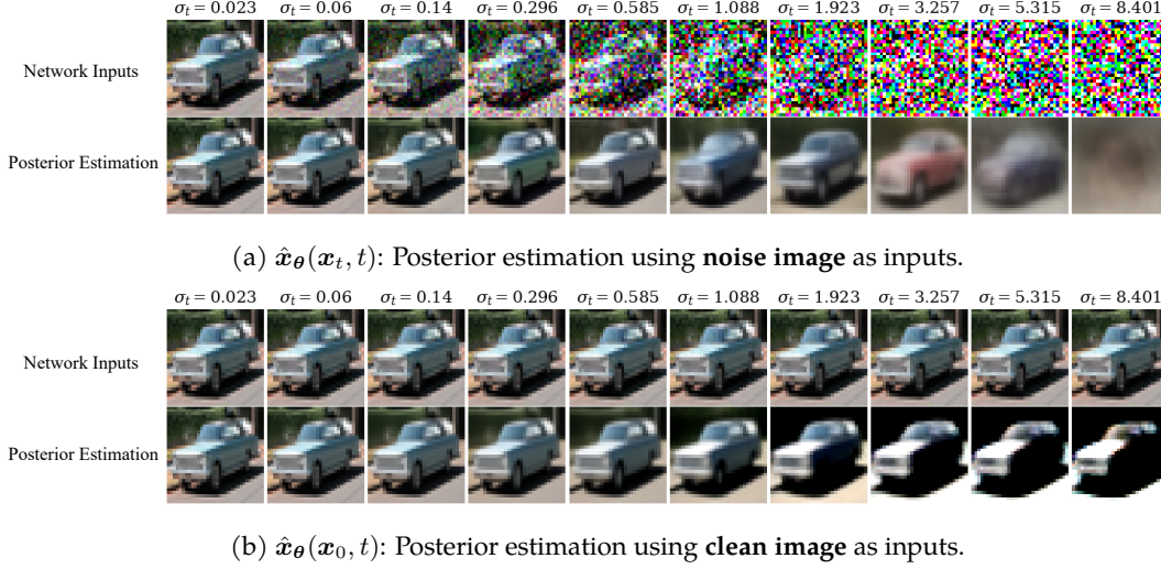
Figure 10: Using clean images as inputs improves posterior estimation quality. We use a pre-trained DDPM diffusion model on CIFAR10 to visualize posterior estimation for clean inputs and noisy inputs across varying noise scales \sigma_t . Clean inputs produce smooth and descriptive estimations even at high noise levels, whereas noisy inputs result in blurry and lossy estimations at large \sigma_t , making it difficult to extract meaningful representations.
