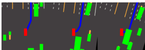
(a) Vehicle without hierarchical planning is out of lane when avoiding collision.
