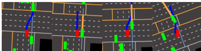
Figure 8: Hierarchical planning enables vehicle re-plan and avoid obstacles adaptively.
