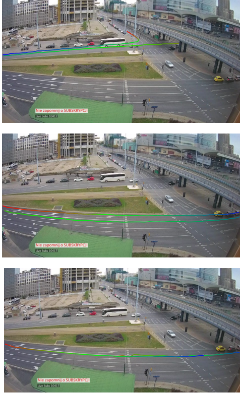
Figure 8: Trajectories selected by multi-object queries. Each image shows two trajectories; the color of each one changes from red to green to blue to denote the progression of time. Top: Unprotected right turn into lane with oncoming traffic, as in Figure 1. Middle: The car on the bottom drives faster than the one on top and passes it. Bottom: One car driving closely behind the other.
