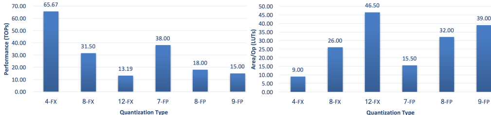
Figure 1: The estimated multiply-accumulate performance on a Xilinx VU9P FPGA, operating at 500MHz, in teraops (left) and area (right) for fixed (FX) and floating-point (FP) in various precisions (both weights and activations).
