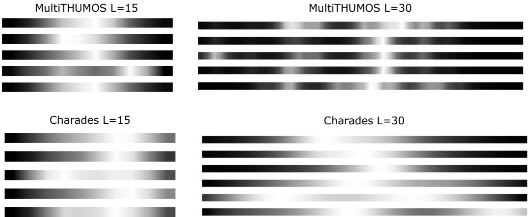
Figure 6: Illustration of several learned TGM kernels. On MultiTHUMOS, it learns to focus on shorter intervals to capture shorter events. On Charades, the Gaussians have a larger \sigma value, resulting in filters that attend to longer temporal durations.
