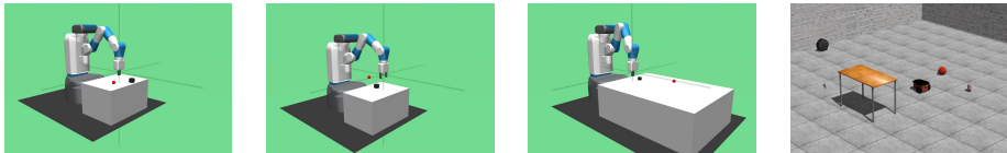
Figure 1: Fetch robot arm environments and a navigation task based on the Gazebo simulator: FetchPush, FetchPickAndPlace, FetchSlide, SocialBot-PlayGround.
