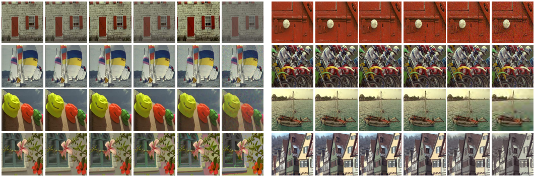
Figure 20: Examples from the TID2013 data set proposed by Ponomarenko et al. (2015). Displayed are a change of contrast, three types of noise, denoising, jpg2000 compression, and two color quantizations (from left to right and top to bottom).
