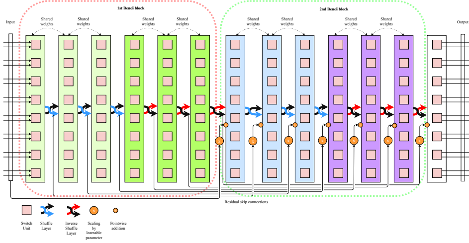
Figure 3: Neural Shuffle-Exchange network with 2 Beneš blocks.
