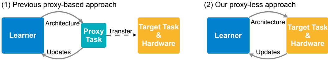
Figure 1: ProxylessNAS directly optimizes neural network architectures on target task and hardware. Benefiting from the directness and specialization, ProxylessNAS can achieve remarkably better results than previous proxy-based approaches. On ImageNet, with only 200 GPU hours ( 200 \times fewer than MnasNet (Tan et al., 2018)), our searched CNN model for mobile achieves the same level of top-1 accuracy as MobileNetV2 1.4 while being 1.8 \times faster.
